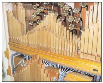
Figure 4. The pipework assembled in the new organ case.
